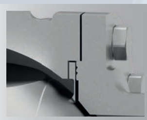
Stellited metal seat ring. Leakage class D according to DIN EN 12266 up to 260°C (500°F).
