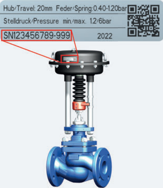
Fig. 3: Name plate showing the ARI-ID and serial number (red box) on a control valve with a pneumatic actuator
